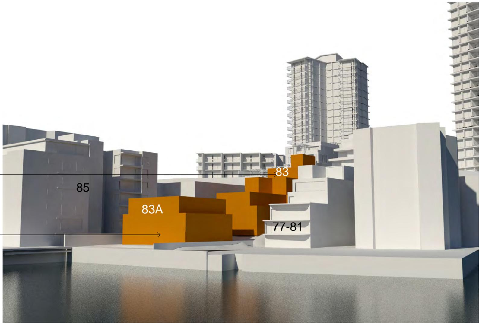
Built form is required to street front boundary to accommodate a 2 storey unit at street level (Lv5 and Lv6), a residential lift lobby and a carpark lift lobby. A lift overrun and motor room are contained in the highest portion of the allowable 9.5m envelope.
